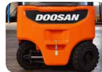
Optimized Steering Angle BT (3-wheel truck): 90° BX (4-wheel truck): 86°
