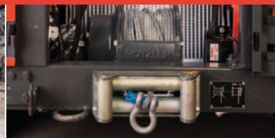
Winch with roller type of rope guides
