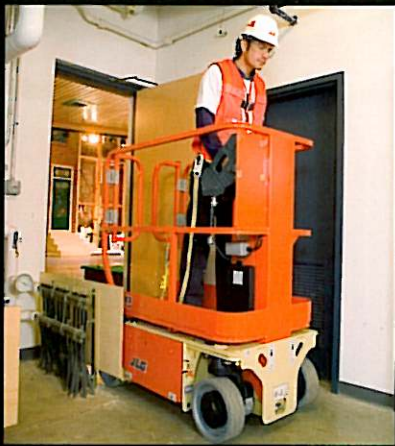
11cm turning radius and narrow profile provides more maneuverability.
