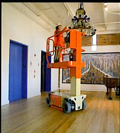
Low overall weight. For use on mezzanine or sensitive floors.
