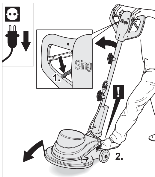
Fig. 16 Release the adjusting lever and carefully tilt the machine back up.
