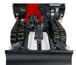
Retracted undercarriage : 980 mm
